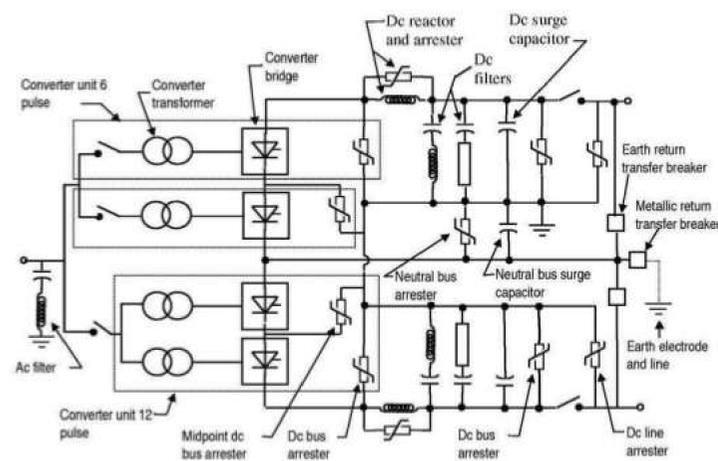
Figure 1: Image of an HVDC system
