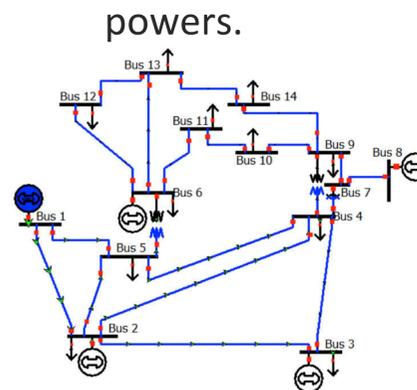
Figure 3: IEEE bus system set up
