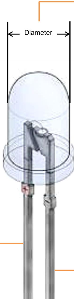
The diameter of an LED refers to the diameter of the case not including the lip at the bottom.
