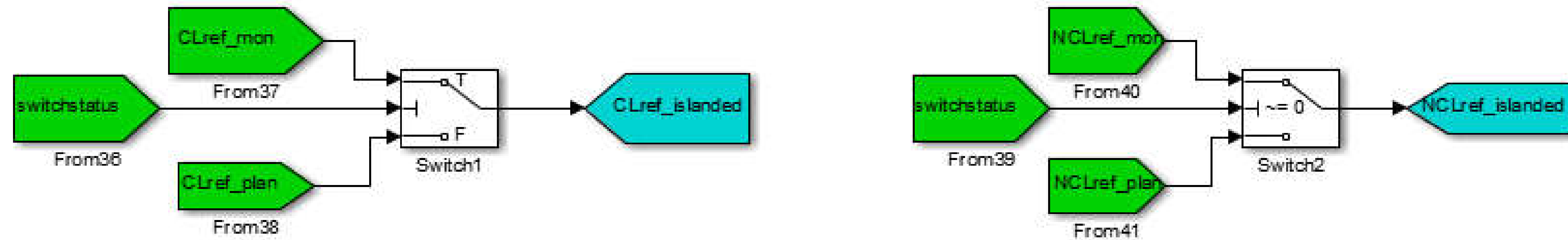
Figure 7. Switches which choose between monitoring and planning block critical and noncritical loads.
