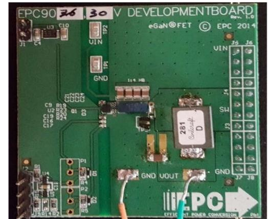
Figure 1: eGaN DC-DC Buck Converter
