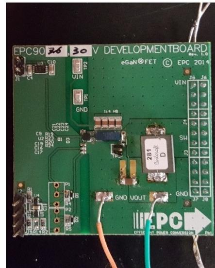
Fig. 1: eGaN DC-DC buck converter
