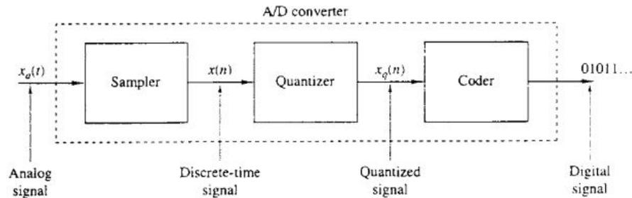
**Figure 4: Process of analog to digital conversion [6]**
