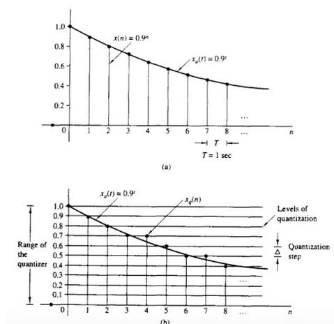
**Figure 8: The graphic describes the process of quantization [6].**
