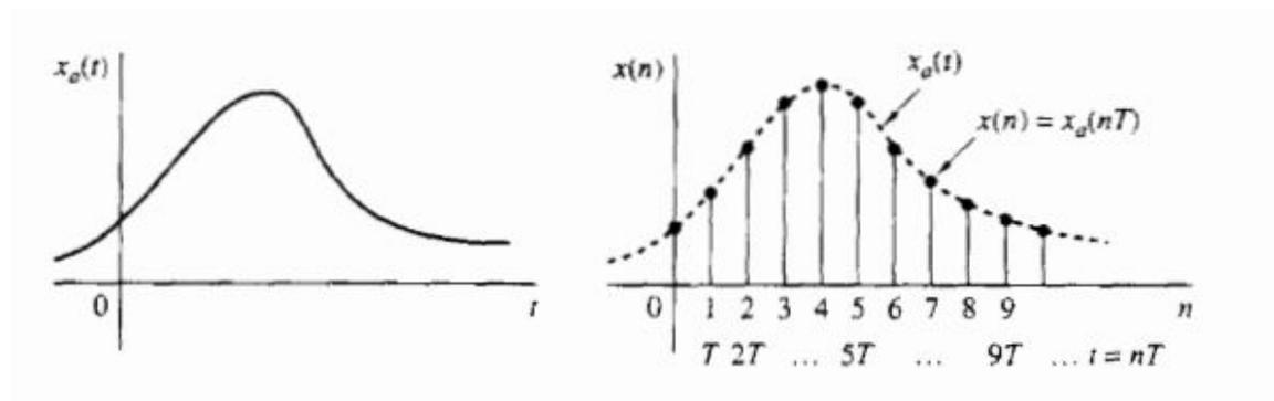
**Figure 5: Process of Sampling [6]**
