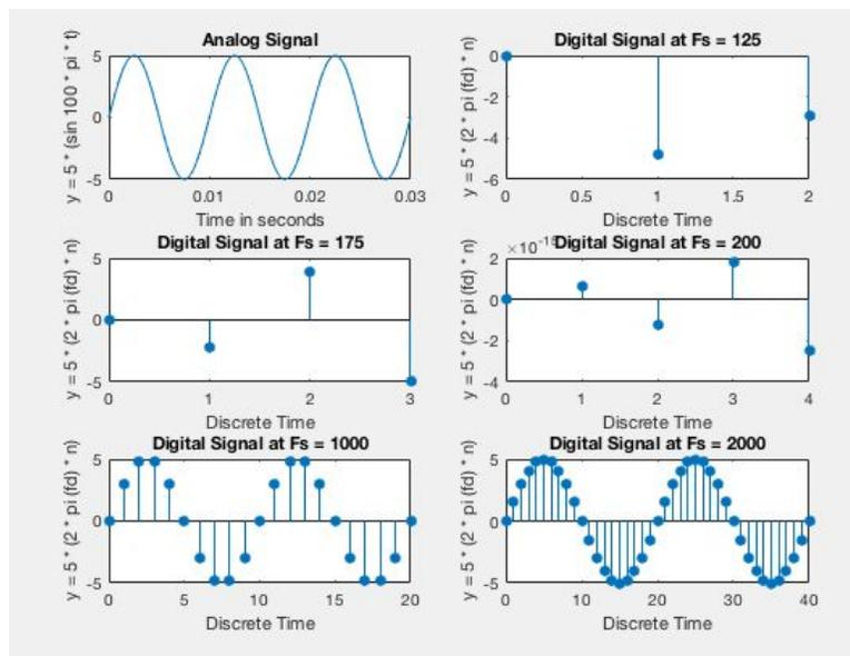
**Figure 6: Testing to the Nyquist-Shannon Sampling Theorem**
