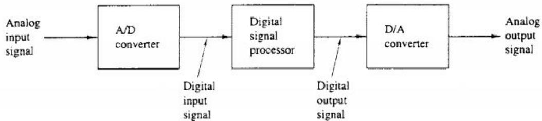
**Figure 3: The process of analog to digital conversion and digital to analog reconstruction [6].**
