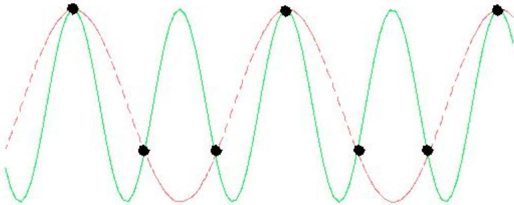
**Figure 7: The green line represents the actual wave; the points represent the sample. Notice that the reconstructed signal (red line) is not the same as the green line [5].**
