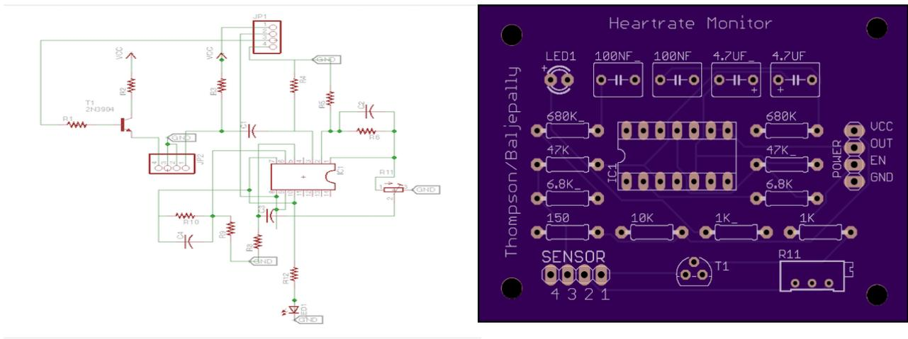
Using the rotation tool, each component was turned in the direction that was requested. In order to connect each of the components, the green wiring tool was used that represents actual wiring on the circuit board. This tool is used to connect the separate ports of each component to the
