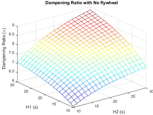
Fig. 3. Dampening ratio when there is no injection from the FESS
