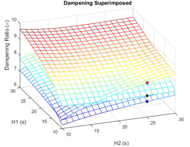
Fig. 4. Dampening Ratio at the various buses. The red marker refers to bus 4, the blue marker refers to bus 9, and the black marker refers to bus 7. In order of top to bottom: Top point is bus 4, Middle point is bus 7, and the bottom point is bus 9.
